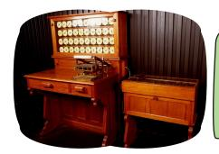
This invention was made in 1890. By this device one could encode the data on the cards with the help of the punched holes. This device was invented by Herman Hollerith.
