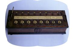
This mechanical calculator was invented in the year 1642 by Blaise Pascal of France. With the help of this calculator one can add, subtract, multiply and divide straightaway by way of replication.
